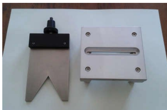
Phot. 1a. Object stage and knife with a triangular notch for Warner-Bratzler texture test (photo L. Lewko)
