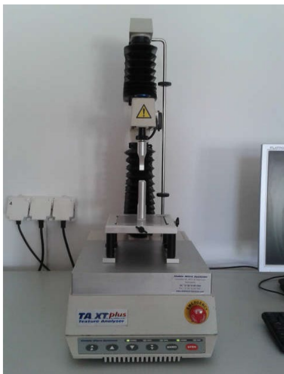
Phot. 1. Test bench – texture analyser TA.XT plus Stable Micro Systems (attachment for measuring the force of biting – Volodkevich bite jaws) (photo L. Lewko)
