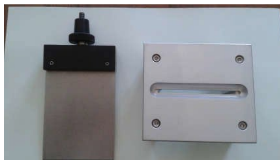
Phot. 1b. Object stage and flat knife for Warner-Bratzler texture test (photo L. Lewko)
