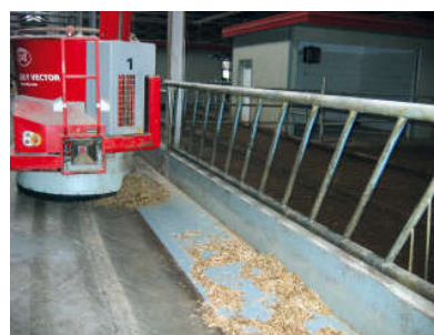
Fot. 3. Robot do mieszania, zadawania i podgarniania paszy Fig. 3. The robot for mixing, feeding and pushing of feed
